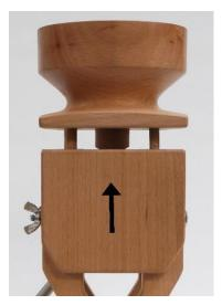
The gear cover can only be removed if the funnel has already been removed. Press the cover slightly upwards with your thumb to lift the pin holder out of the slotted holes. The cover can be removed towards the front.
